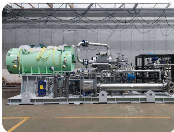
Petrochemical PTA Reactor Feed Pump Skid
